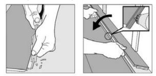
Remove the raised edge of the click connection as shown in the image above. Use suitable adhesive for attachment where necessary. Place spacers between the last floor panel and the wall until the adhesive has cured.
