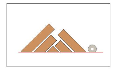
When we reach the last strip, the cut floorboards from the first row (step 3) come in handy again. The remnants of the first row's triangles can be used to fill in the remaining gaps and complete the floor.
