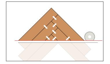
3 Cut the triangle along the red line as indicated in the image next to it. This is a starter triangle. The remaining planks below the red line can be used later for the final row. Ensure that all starter triangles are the same, with three planks on the left side of the triangle and two on the right side, as shown in the example above. Avoid having starter triangles with three planks on the right side and two on the left side.
