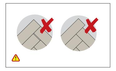
2 Attention! Installing a dryback floor requires some precision. The smallest allowable gap will repeat and become larger as the floor is further laid. Be meticulous about this for the best result.
