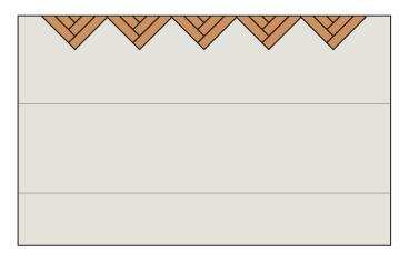
Also, secure the triangles on the left and right sides to the underlayment in the same way. By placing the protective film back over the triangles, the adhesive layer remains protected. Ensure that the exposed adhesive layer does not get contaminated, as this can reduce its adhesive quality. Avoid walking or kneeling on the exposed adhesive layer at all times.
