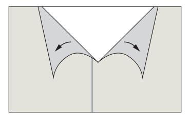
Place the first triangle on the self-adhesive underlayment so that the installation line aligns exactly with the centerline. To do this, gently peel back the protective film from the underlayment and make a small cut along the centerline.
