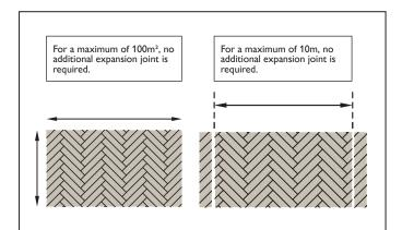
The maximum area to be installed is 100 m<sup>2</sup>. The maximum length of the floor surface that can be laid in one direction is 10 m. For an area larger than 100 m<sup>2</sup> or a length greater than 10 m, an additional expansion joint is required. Additionally, all expansion joints along the walls must be increased by 5 mm.
