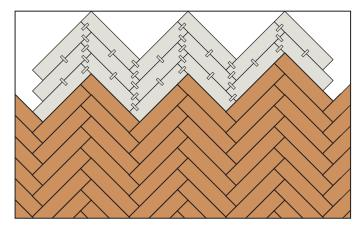
S Repeat this procedure on the left and right sides of the laid starting strip. Continuously check if all the corners are still 90°.
