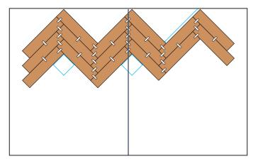
Place the attached strips against the starting wall, with the points aligned with the centerline as shown in the image next to it. Check if all the corners are 90° and if the distance to the starting wall is consistent throughout.
