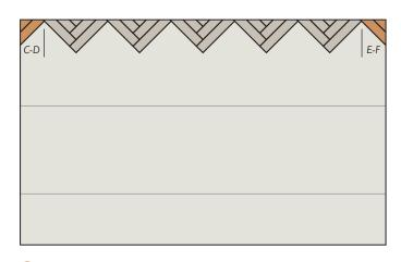
Fill in both sides. Cut distances C-D and E-F of the last triangle, and place it. The PVC Dryback pieces can be easily cut to size with a utility knife.
