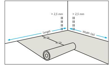
The self-adhesive underlayment can be easily cut to size with a utility knife. Place the underlayment along the width (W) of the room with the protective film facing up. Ensure that there is a 2.5 mm gap between the underlayment and the wall. To prevent the underlayment from shifting, secure the strips together with tape.
