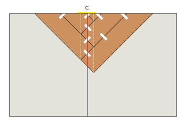
Place the first triangle in such a way that the installation line of the herringbone pattern aligns exactly with the centerline of the room. Use the marker (C) to verify this.
