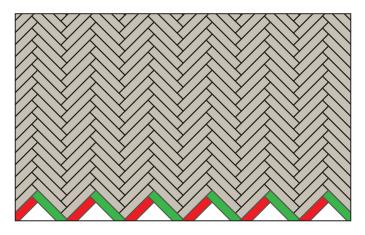
Continue laying the entire space in this manner. After 30 minutes from installation, the floor can be lightly loaded. This allows kneeling on the floor to install other PVC Dryback parts.
