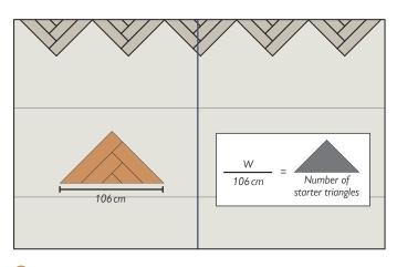
To determine the number of triangles needed, you will require the total width of the installation side. Divide this width by 106 cm (the longest side of the triangle).
