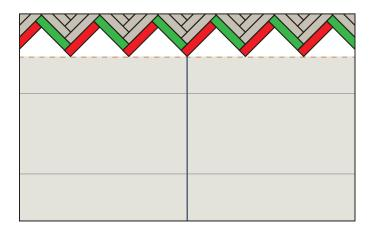
13 There is a maximum of 10 minutes to move incorrectly installed planks. However, do not do this too often (no more than 2 times), as it reduces the adhesive capability of the underlay. Do not load or put weight on the planks immediately after installation. The centerline should always be visible. Ensure that the straightness (the orange dotted line) remains straight in relation to the room at all times.
