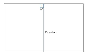
Determine (from the perspective of the starting wall) the center of the room. Use a chalk line to create a line perpendicular to the starting wall and pull it tightly. This is the centerline.
