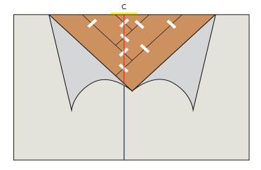
Peel back the protective film to the size of the starter triangle and place the first triangle on the self-adhesive underlayment.
