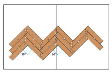
2 Lay two to three rows of strips next to each other. Ensure that the corners are perfectly 90° and secure the corners together with tape.
