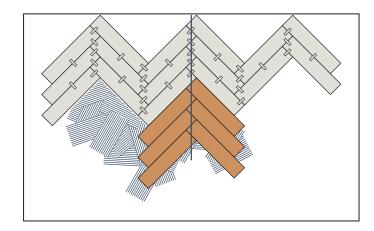
Follow the recommended guidelines for adhesive consumption, waiting time, and setting time. Use the notched trowel to spread the adhesive. Apply adhesive to the floor in a width that accommodates two or three strips (the dark strips in the image) and place these strips in the adhesive. The floorboards should be rolled immediately after laying the adhesive. Always do this within the specified working time of the adhesive.
