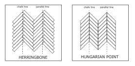
The point of the pattern should connect to the chalk line accurately. When the first row of floor panels in the room has been laid, it will serve as a mould for the remaining following rows on the left and right side.
